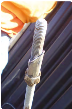
For particularly hard soils, adding a custom collar to the drive rod can prevent the rod from punching through the anchor.
