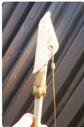
For particularly hard soils, adding a custom collar to the drive rod can prevent the rod from punching through the anchor.
