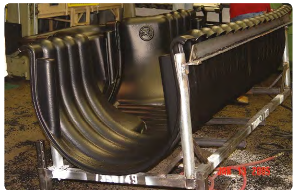
SmartDitch semi-circular tee-section channel in trim fixture.
